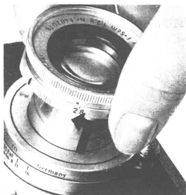
Catch locking the lens at the infinity setting
